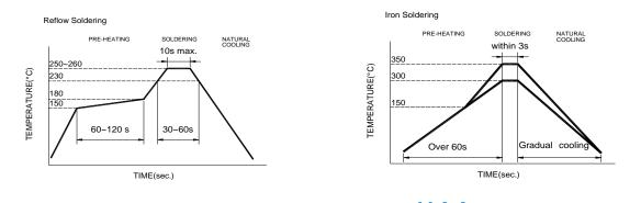
Recommended temperature profiles for re-flow soldering in Figure 1.
