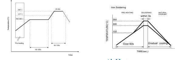
Recommended temperature profiles for re-flow soldering in Figure 1.
